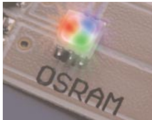
By using 3 diodes in one LED package, color mixing is achieved without color separation.
